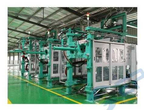
Shape Moulding Machines and Aluminum Moulds are the major processor of Shape Moulding Plants.  We engineered all machines our by latest technology for best quality products and also our all equipment are fully automated and shape moulding machines have individual vacuum pumps.
